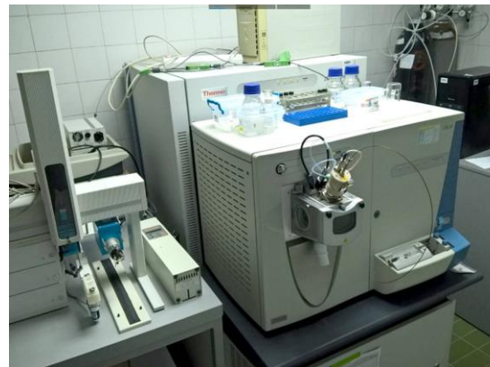
Thermo ESI-MS LTQ ORBITRAP High Res. m/z 1:100.000 with linear ion-trap FT (quadrupole) MS/MS, MS n
