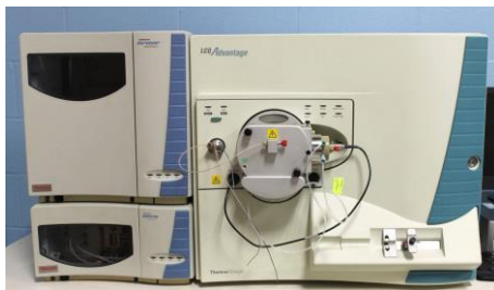
Thermo ESI-MS Advantage with ion-trap MS/MS, MS n
